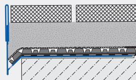
Installation in drainage mortar/gravel/chippings with plug-in profile
