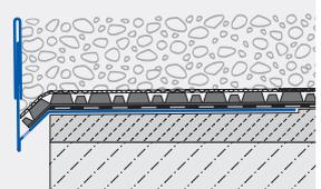
Installation as a gravel strip with plug-in profile
