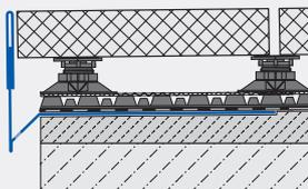
Installation on supports with plug-in profile
